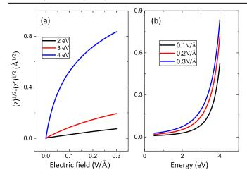
FIG. 4 (color online). (a)  $(z)^{1/2} - (z')^{1/2}$  as a function of the electric field at different energies. (b)  $(z)^{1/2} - (z')^{1/2}$  as a function of energy at different electric fields.
