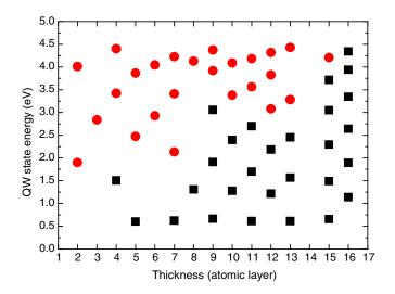
FIG. 3 (color online). Energies of quantum-well states at 0.1 nA versus island thickness. The energy shifts of quantum-well states behaving like the first (second) mode are marked by circles (squares).
