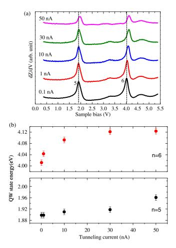
FIG. 1 (color online). (a) dZ/dV-V spectra acquired on the island with a thickness of two atomic layers under set tunneling currents of 0.1, 1, 10, 30, and 50 nA. The peaks of quantum-well states in the spectrum are marked by quantum numbers 5 and 6. Dashed lines mark the peak energies at 0.1 nA. (b) The energies of two peaks as a function of tunneling current, showing a monotonically positive energy shift.
